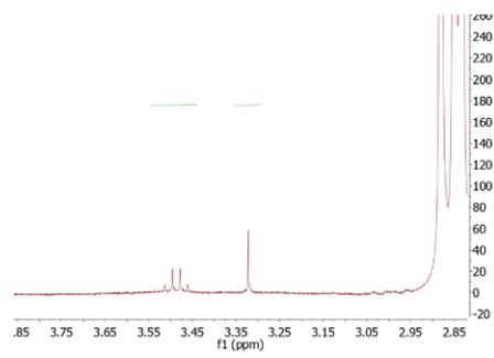
Figure 12 – CH<sub>3</sub>OH and Et<sub>2</sub>O (?) residue in ZEN
