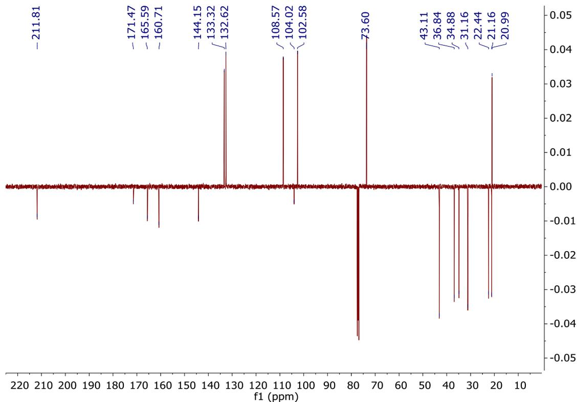
Figure 5 – APT spectrum of ZEN. Down = CH<sub>2</sub>/C<sub>q</sub>; Up = CH/CH<sub>3</sub>.
