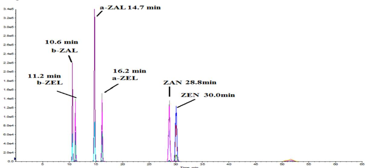
Figure 9 TIC chromatogram of the standard mixture.
