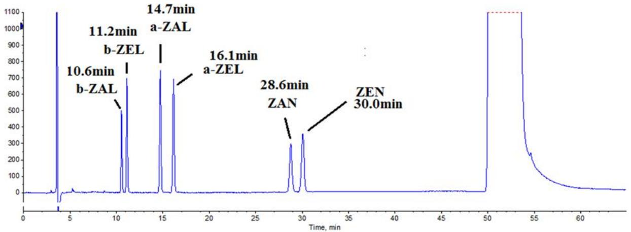
Figure 7 – Chromatographic separation of the test mixture with LC-DAD detection
