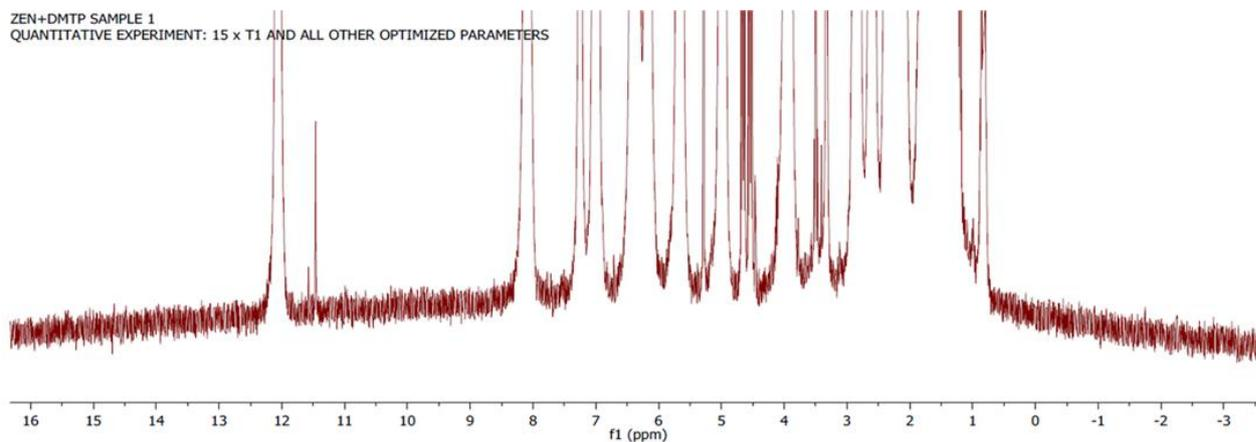
Figure 14 - NMR spectrum of ZEN in  $\text{CDCl}_3$
