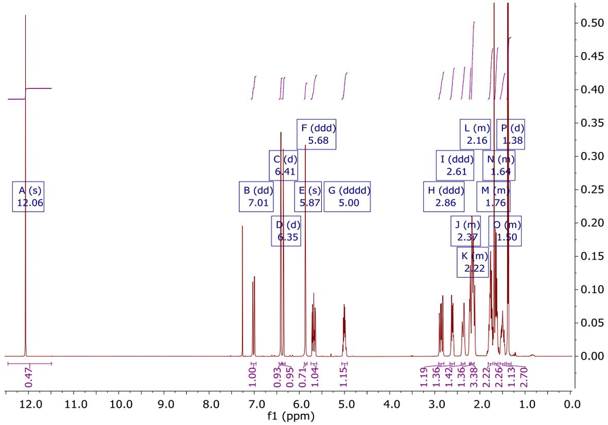
Figure 3 – <sup>1</sup>H NMR spectrum of the ZEN in CDCl<sub>3</sub>.
