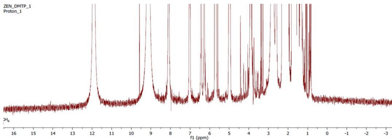
Figure 15 - NMR spectrum of ZEN in acetone- $\text{d}_6$
